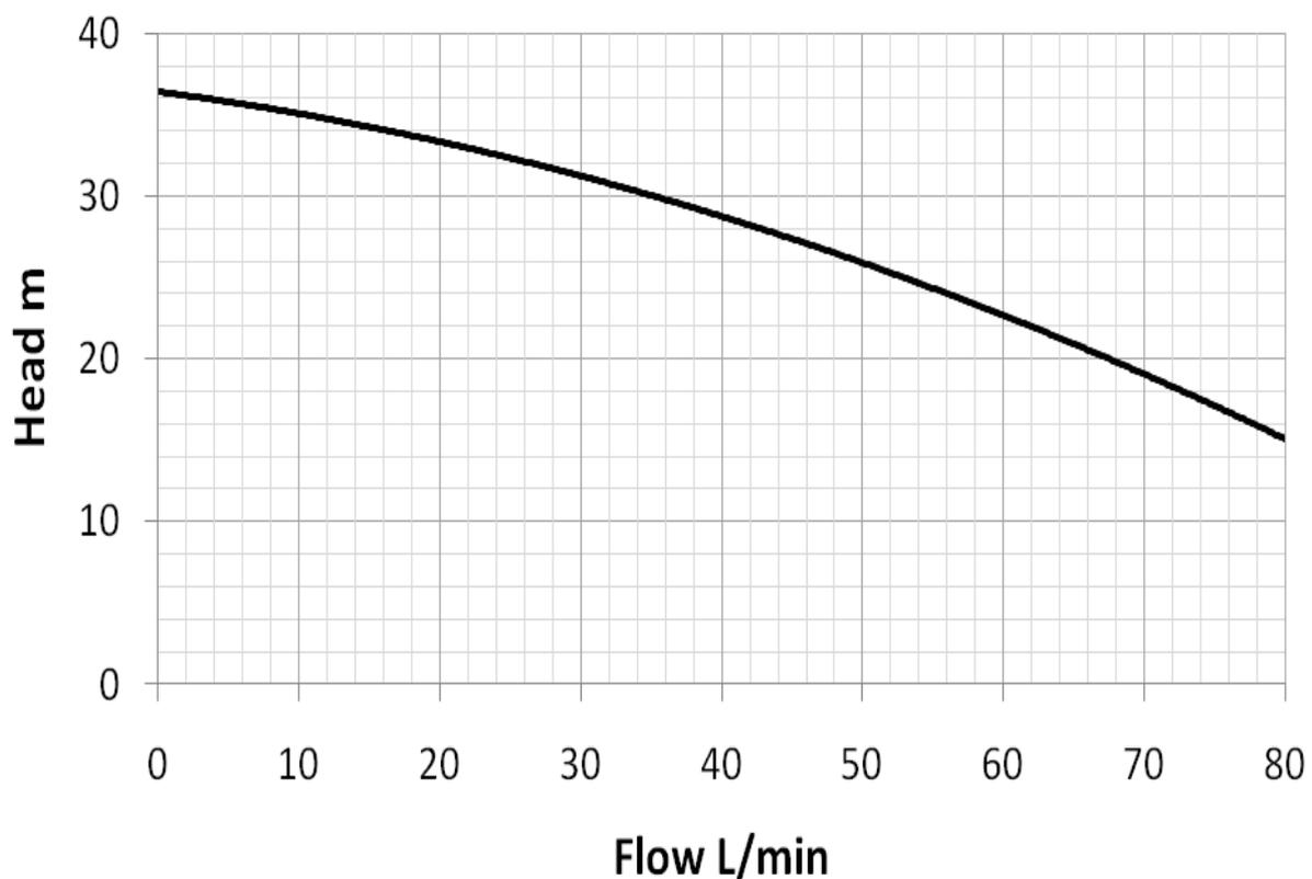
Figure 2 Pedrollo NKm 2/1 characteristic curve (power 0.45 kW)
