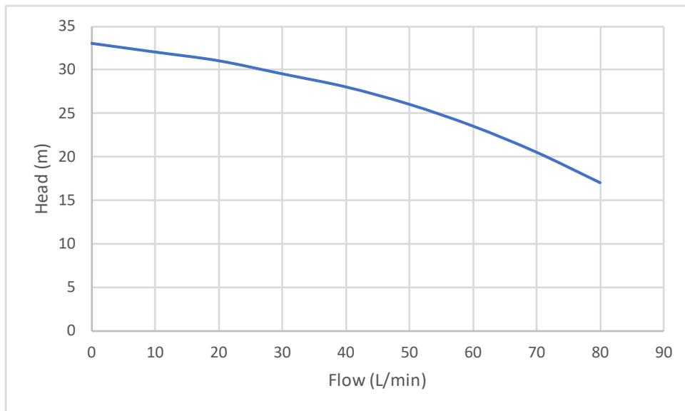
**Figure 2** Pedrollo NK 2/2-N characteristic curve (power 0.37 kW)
